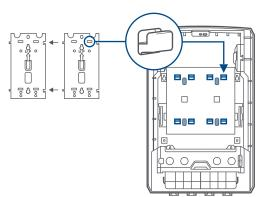
**Direct Mount:** Position unit on wall so that the top is level. Use key to open front cover and mark screw locations where indicated with circles. Secure unit to wall with four anchored screws appropriate to the type of wall in locations previously marked.
